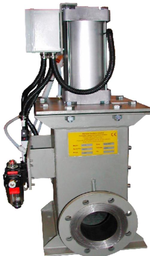
The **Series Diverter Valve** is a very convenient method of distributing material into multiple reception locations in a pneumatic conveying system. It is mounted onto the top of the reception hopper or silo connected to a simple rectangular flange.
