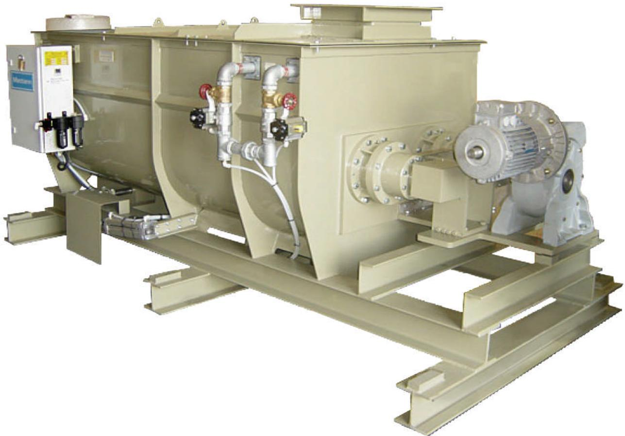
The Macawber **Ash Conditioner** thoroughly mixes fly ash with water in a controlled way. The unique control arrangement imposes regulation to both ash volume and to water volume to ensure that the conditioned ash is neither too wet nor too dry.
