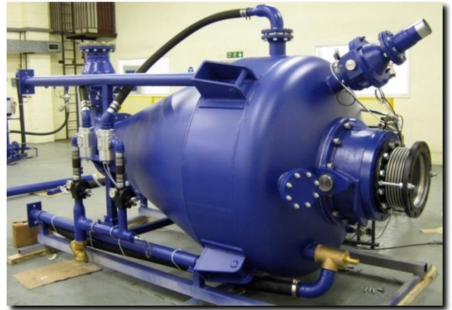
System 3 conveying vessel during assembly.
